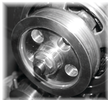
8. Install the Serpentine Alternator pulley. Be sure to face the raised hub outward.
