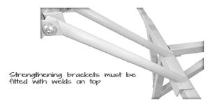
5. The top and base of the seat can now be joined together. This is done by sliding the seat frame over the triangular bracket on the seat base.
